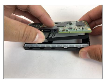
Lift the motherboard up from the bottom.
