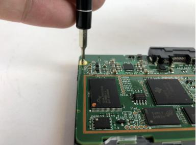
Remove the three 5.4mm JIS #00 screws from the motherboard.
