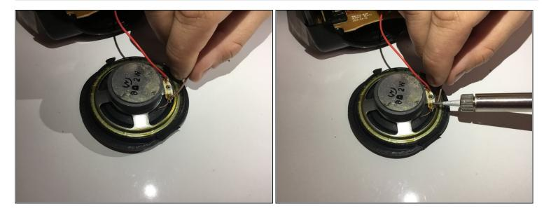
• Soldering will be required to install the wires to your new speaker.
