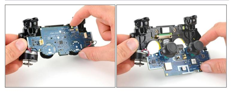
A Be careful not to strain the vibration motor cables. <u>Follow this guide</u> to re-solder the vibration motors if they break off the motherboard.
