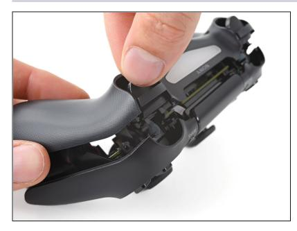
• Press the L2 button and slide the rear case over it.
