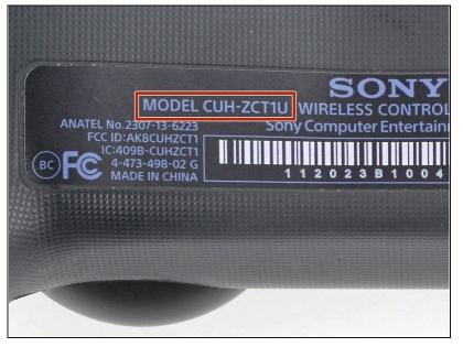
Check the model number on the back of your controller. This guide was written using model CUH-ZCT1U. If you have another model, the guide procedure and replacement parts may differ slightly.
