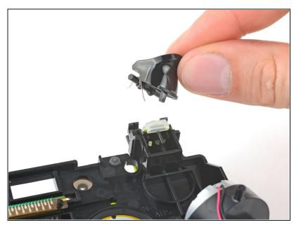
• Unclip the L2 button from the midframe and remove it, making sure not to lose the small spring from the inside peg.
