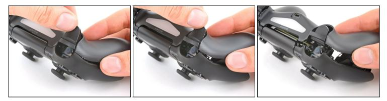
• Press the R2 button and slide the rear case over it.
