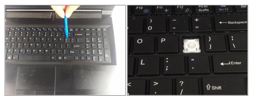
• Using a plastic opening tool, gently pry the key up.
