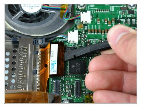
Use the flat end of a spudger to pry the PC card cage cable connector up off the logic board.
