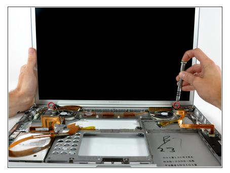
While supporting the display with one hand, remove the last two T6 Torx screws from the display hinges.
