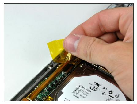
• If necessary, remove the strip of tape covering the speaker cables.
