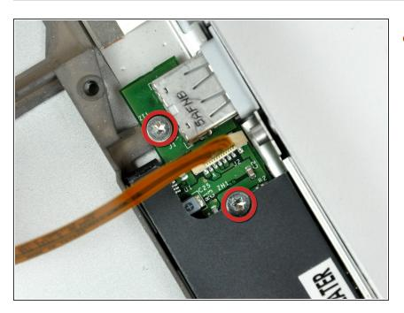
Remove the two T8 Torx screws securing the PRAM battery & USB board to the lower case.
