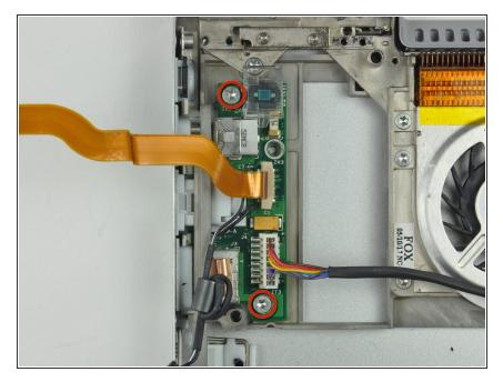
Remove the two T8 Torx screws securing the DC-in board to the lower case.
