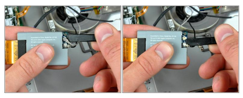
• Use the flat end of a spudger to pry both antenna connectors off the AirPort/Bluetooth board.
