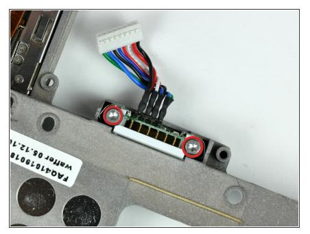
Remove the two 8.5 mm T8 Torx screws securing the battery connector to the lower case.
