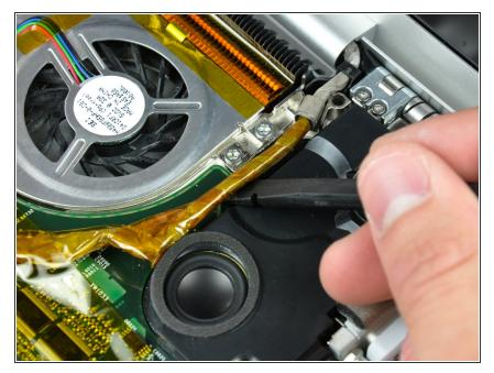
• Use a spudger to de-route the display data cable from the channel in the right speaker.
