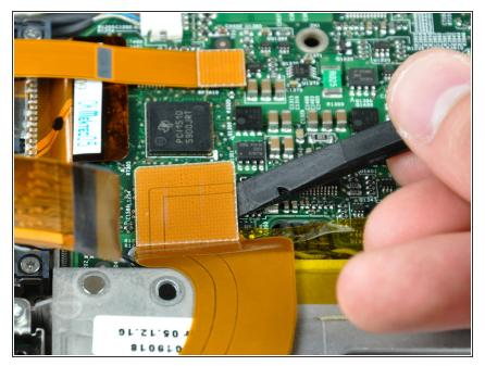
• Use the flat end of a spudger to pry the sound card cable connector up off the logic board.
