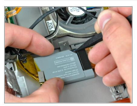
Use the tip of a spudger to press the metal pressure connector down through the hole in the AirPort/Bluetooth board and lift it out from the lower case.
