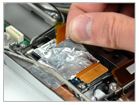
Peel back the piece of foil tape covering the modem cable to free the speaker cable held underneath.
