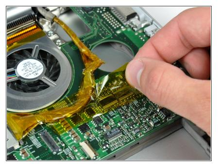
If necessary, remove the piece of tape securing the display data cable to the logic board.
