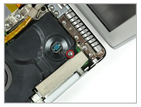
Remove the single T8 6.9 mm Torx screw securing the right speaker to the lower case.
