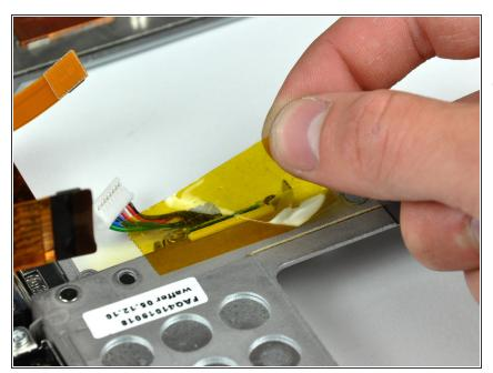
*i* If necessary, remove the strip of yellow kapton tape covering the battery connector.
