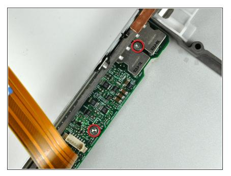
Remove the two T8 Torx screws securing the sound card to the lower case.
