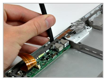
• Use the flat end of a spudger to pry the USB sockets away from the left edge of the lower case.
