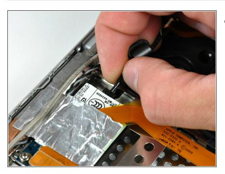
Disconnect the RJ-11 cable from the modem.
