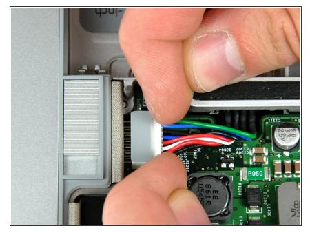
• Disconnect the battery cable connector straight away from its socket on the logic board.
