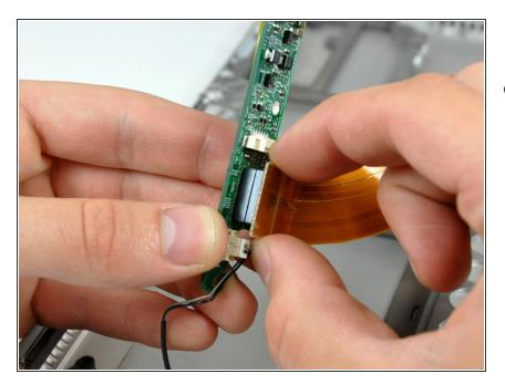
Pull the sound card ribbon cable straight away from its socket on the sound card.
