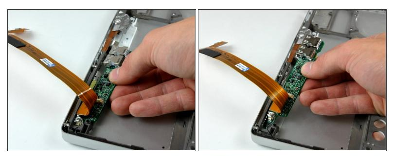
• Lift the sound card slightly out of the lower case, minding the fragile lower portion holding the microphone connector.
