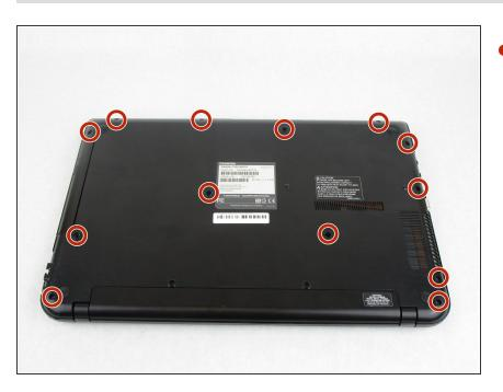
Use a Phillips #1 screwdriver (PH1 bit) to remove the thirteen 7 mm screws that secure the bottom cover.
