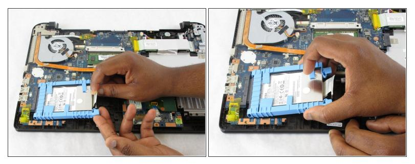
• Using the ribbon beneath the hard drive lift it upwards and pull the hard drive out.
