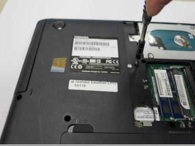
Using a Phillips #0 screwdriver, remove the single 3mm screw.
