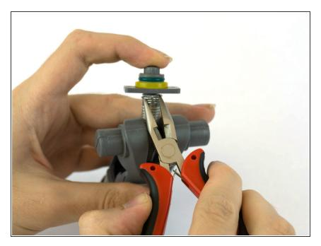
• Use needle nose pliers to compress metal clamp .
