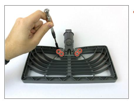
Remove the four 10mm screws holding the joint assembly to the mop head with your Phillips #2 screwdriver.
