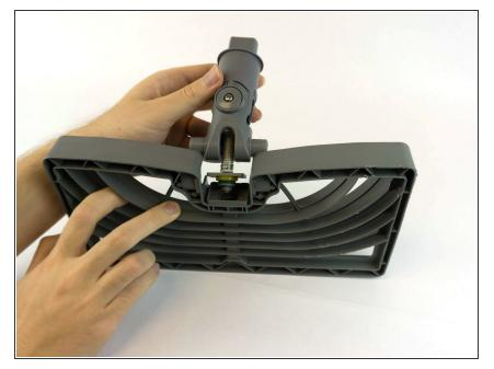
Lift joint assembly out of hinge socket and pull upward with mild force to disconnect steam nozzle.
