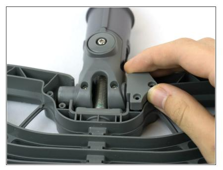
Remove the two plastic hinge covers by pulling the hinges out of the joint and sliding the covers off.
