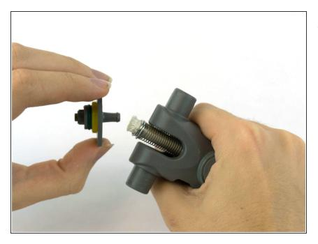
• Pull the nozzle out of the tube.
