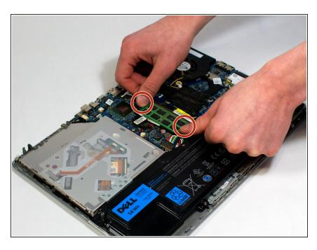
Carefully pull on the tabs on either sides of the RAM.
