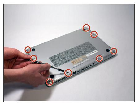
Remove the back cover of the laptop by unscrewing eight 3.5mm screws using a Phillips #0 screwdriver.
