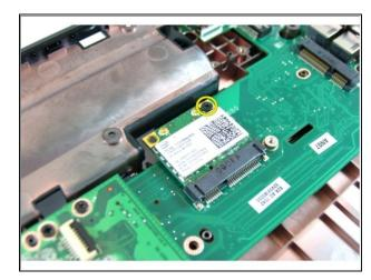
• Remove the screw that secures the WLAN card.
