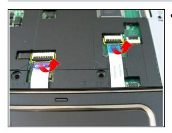
• Release the latches on the system board connector, then disconnect the touch pad cable and the finger printer cable.
