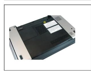
• Loosen the screw that secures the memory door.
