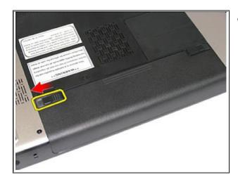
• Slide the left and the right battery release latches to the unlock position.
