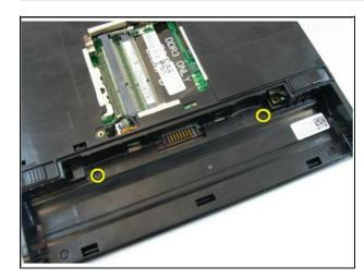
• Remove the screws in the battery compartment.
