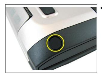
• Remove the rubber from the bottom base on the right side.
