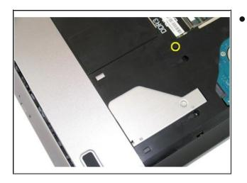
• Remove the screw that secures the optical drive to the computer.
