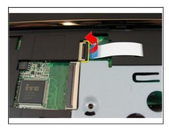
• Release the latch on the system board connector and then disconnect the hot key cable.
