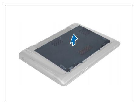
Lift the cover upwards and away from the computer.
