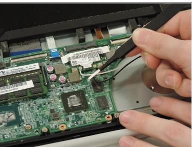
Remove the black and white wires connecting the fan to the network adapter.
