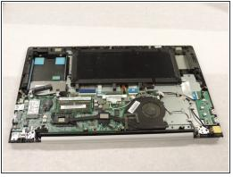
Use a pry tool or iFixIt Opening tool to separate the back panel from the device.
