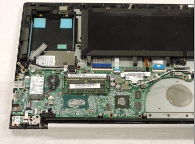
Lift the fan straight out of the casing.
