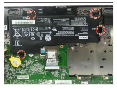
Remove the four 4mm screws on the battery.
