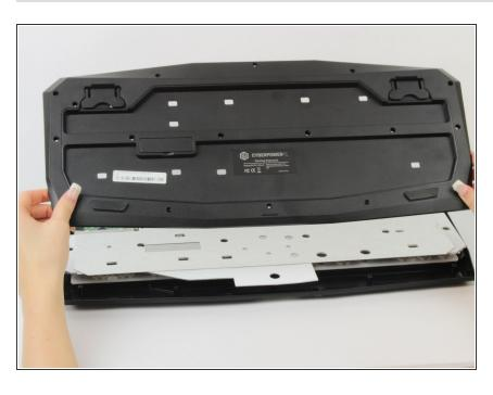
Lift up and remove the plastic casing.
