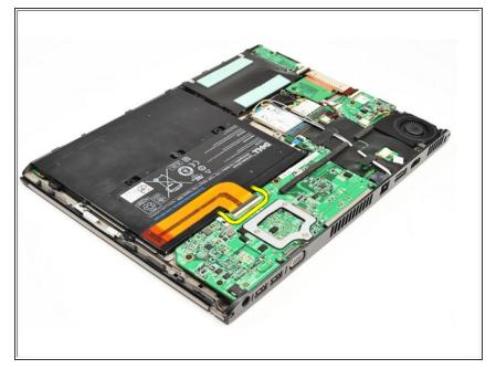
Lift the black cable-release clip to release the battery cable from the connector on the system board and disconnect the battery cable.
