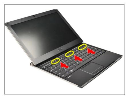
Starting on the right side of the system, use a plastic scribe to pry up the LED cover from the computer.
