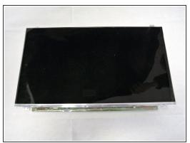
Peel the tape off the cable connected to the back of the LCD screen and unplug the cable which is connected to the bottom. The screen should now be fully removed from the laptop casing.
