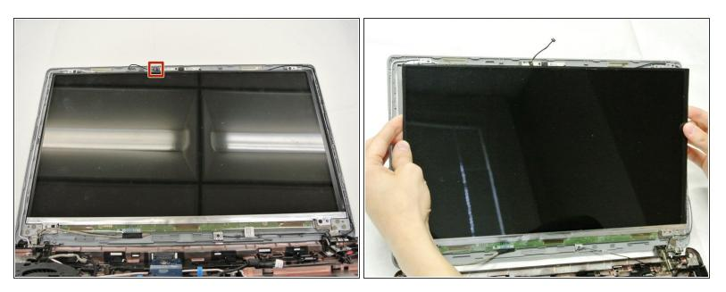
Unplug the black cable connected to the webcam above the LCD screen.
