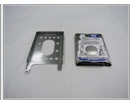
Remove the two 9.0 mm screws on each side of the silver box to slide the hard drive from the silver box housing.
