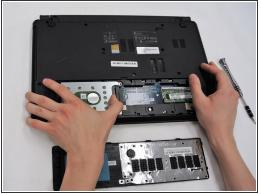
Remove a single 9.0 mm screw on the silver box containing the hard drive. Pull the plastic flap at the side opposite to the side of the screw housing back in order to remove the silver box containing the hard drive.
