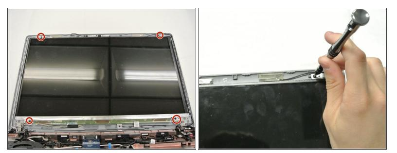
Use a PH0 Phillips head to remove four 3.4mm black screws. Remove the screen from the casing before moving on to the next step.
