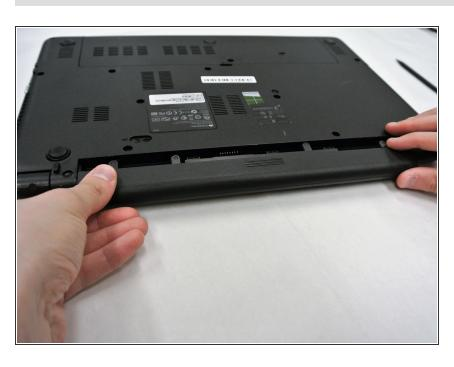
Pull the battery out, making sure to pull the battery parallel to the device.
