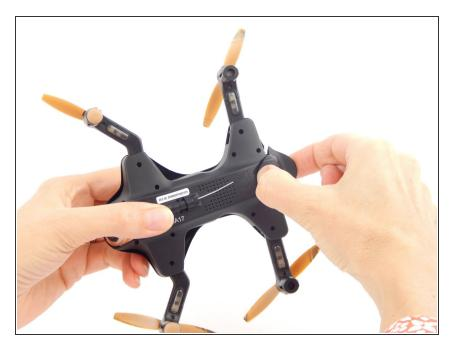
Grasp the tail end of the drone where the lip of the battery protrudes.
