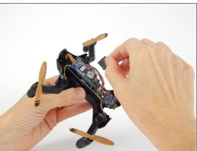
Remove the foam adhesive pad located on the Wi-Fi transmitter board.
