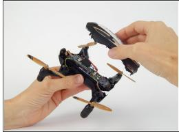
Flip the drone over and lift off the top plastic shell of the drone.
