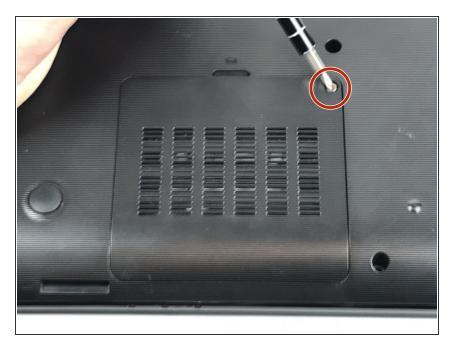
Unscrew the single Phillips #0 screw from the RAM panel.
