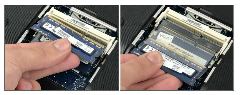
Lift the RAM module to an angle of about 30 degrees and slide it out.
