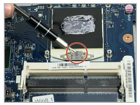
Rotate the lock 90 degrees using a Torx T8 in order to remove the processor.
