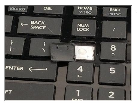
If there is any debris underneath key, first clean before replacing it.
