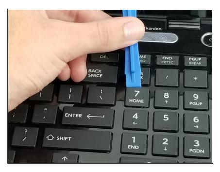
Using the plastic prying tool, slide the edge of the tool underneath the selected key and pry upwards
