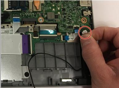
• Disconnect the small wires attached to the top of the right side speaker as marked in the photo.
