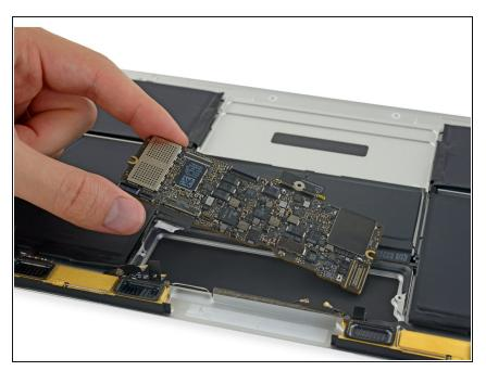
• Remove the logic board.
