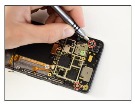
Remove the two 2.5 mm PH00 screws.
