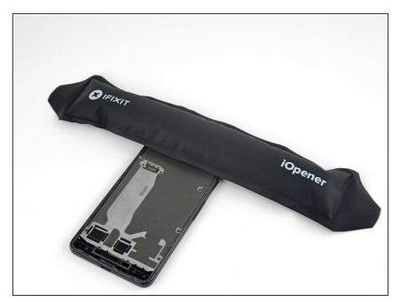
Apply a <u>heated iOpener</u> to the proximity sensor on the top edge of the midframe for two minutes to soften its adhesive.
