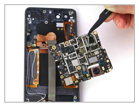
Remove the motherboard by lifting gently out of the device.
