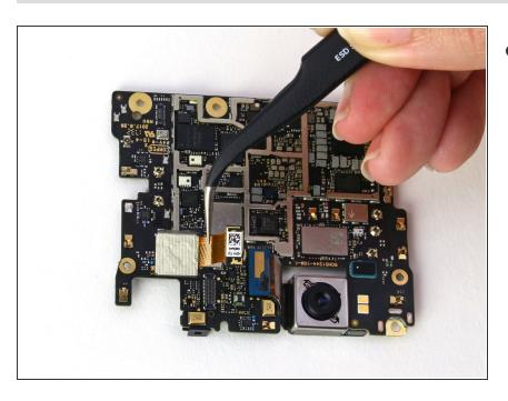
Remove the front camera from the device.
