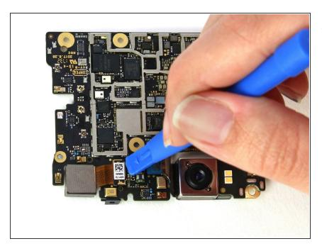
Use a plastic opening tool to disconnect the front camera's press fit connector
