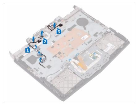
Remove the display cable from the routing guides on the palm-rest assembly.
