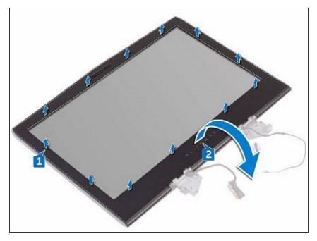
Align the display bezel with the display back-cover and antenna assembly and gently snap the display bezel into place.
