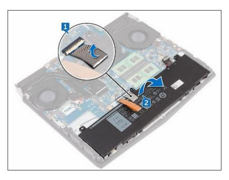
Adhere the keyboard connector that secures the battery to the palm-rest assembly.
