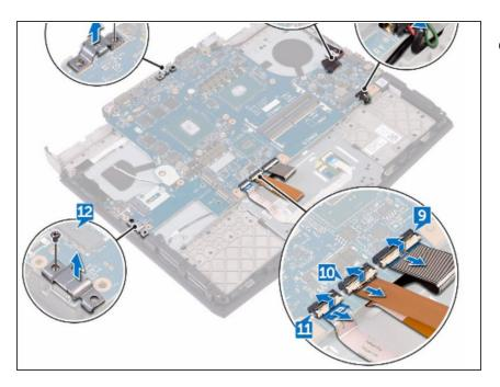
Disconnect the speaker cable from the system board.
