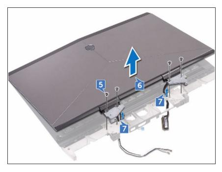
Remove the cables from the routing holes on the palm-rest assembly.
