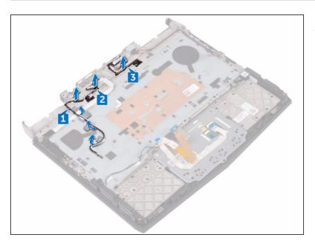
Route the antenna cables through the routing guides on the palm-rest assembly.
