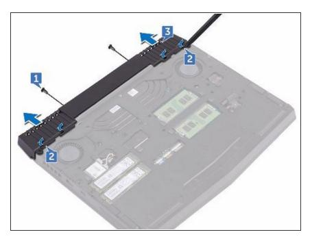
Slide the **NEW** rear-I/O cover into the slots on the computer base and snap the rear-I/O cover into place.
