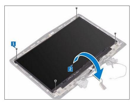
Replace the four screws (M1.6x2) that secure the display panel to the display back-cover and antenna assembly.
