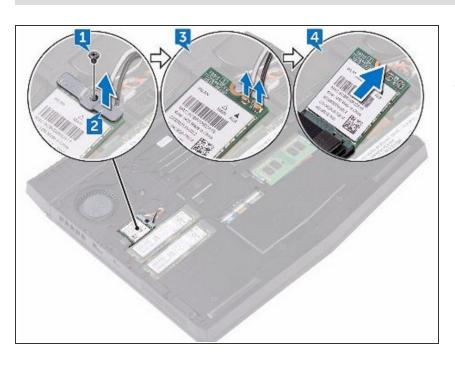
Lift the wireless-card bracket off the wireless card.
