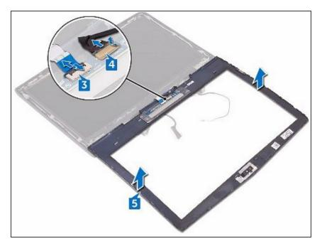
Lift the display bezel off the display assembly.
