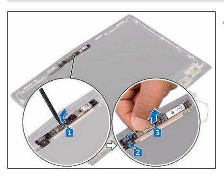
Lift the camera module from the display back-cover and antenna assembly.
