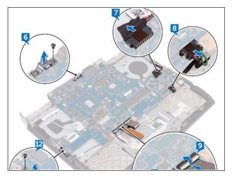
Open the latch and disconnect the keyboard-backlight cable from the system board.
