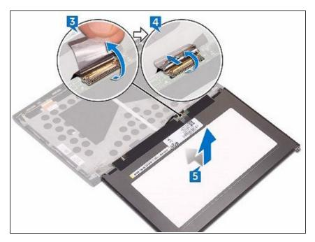
Lift the display panel off the display back-cover.
