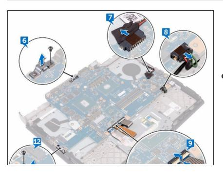
Align the screw hole on the USB
