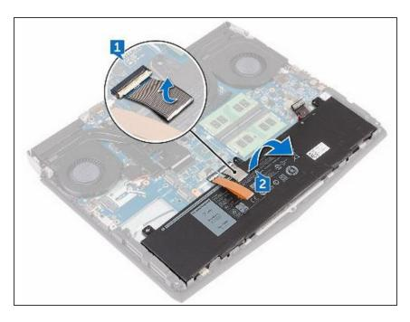
Lift the battery off the palm-rest assembly.
