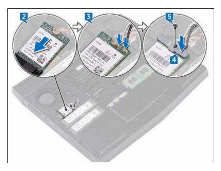
Replace the screw (M2x3) that secures the wireless-card bracket to the wireless card and the computer base.
