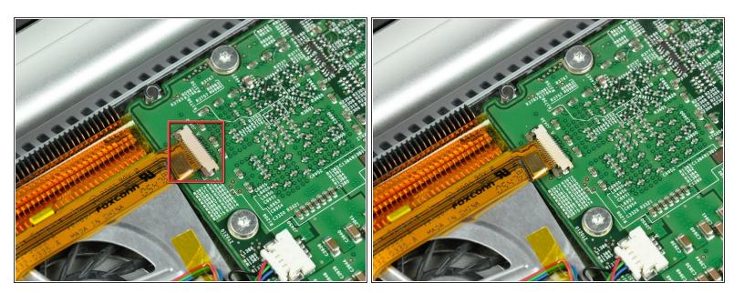
• Use your fingernails or the tip of a spudger to separate the ZIF cable lock from its socket.
