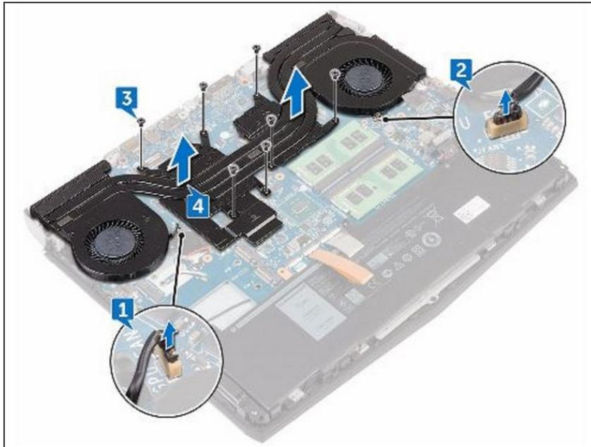
**⚠ CAUTION:** Incorrect alignment of the heat sink can damage the system board and processor.
