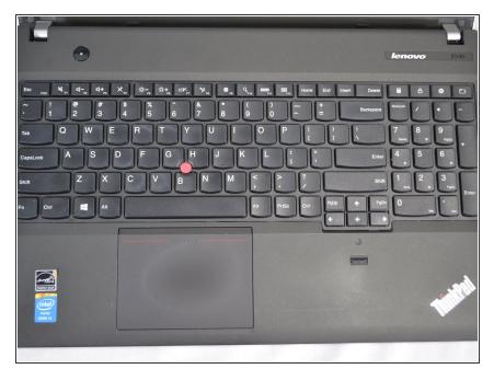
Push the keyboard forward towards the display to create a gap above the trackpad.
