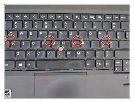
Remove the four 1mm Phillips #00 screws found hidden underneath the keys.
