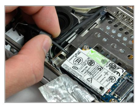
Disconnect the RJ-11 cable from the modem.
