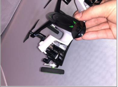
Use the opening tool to separate the drone's body from the drone's shock absorber.
