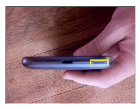
Remove back plate starting with this tab
