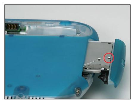
Remove the single black Phillips screw from the center of the CD-ROM bezel.
