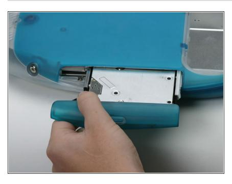
Grasp the CD-ROM bezel and rotate it upward to remove it from the drive.
