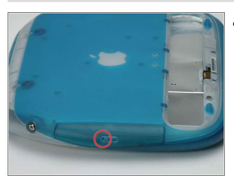
Use a straightened paperclip to manually eject the CD-ROM tray.
