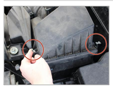
After you have replaced the new filter, close container and latch both metal hooks to close the container.
