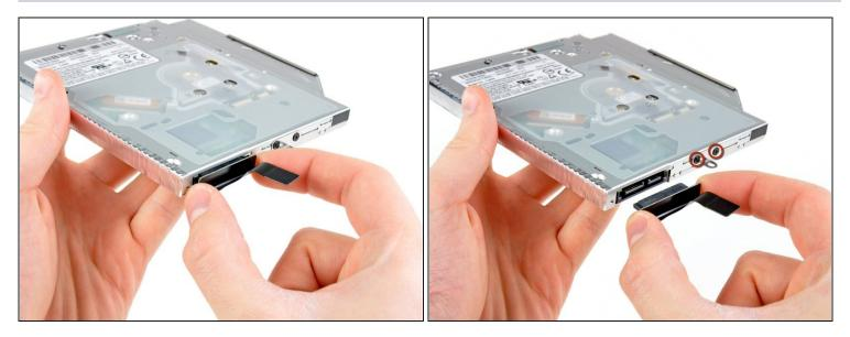
• Pull the optical drive cable away from the optical drive.
