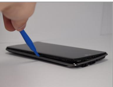
Use a plastic opening tool to separate the screen from the outer frame.
