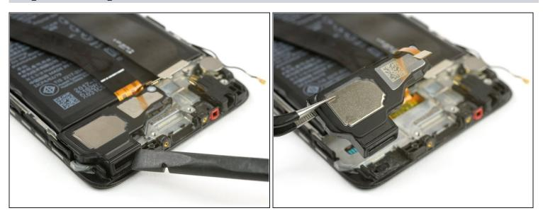
$\triangle$  Only insert the spudger as deep as 1/16 of an inch to avoid damage.
