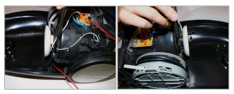
• Unscrew the top two screws on the vacuum.
