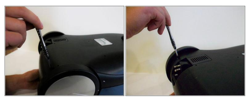
• Unscrew both screws near the wheels.
