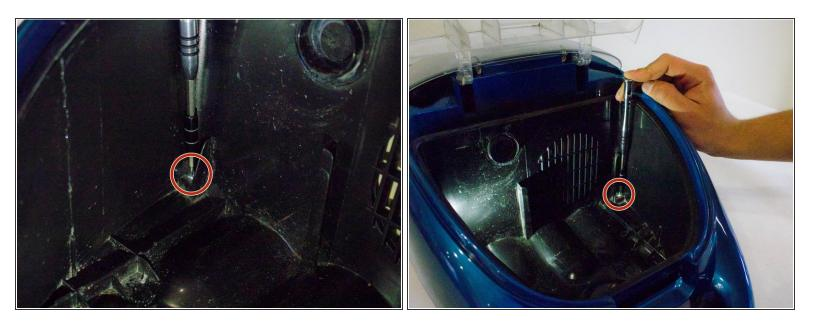
Unscrew the two screws underneath the dirt collection box inside the vacuum.
