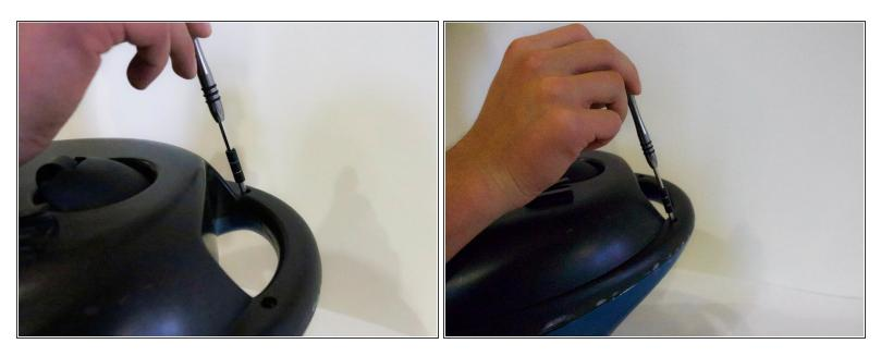
• Unscrew both screws on the bottom of the handle.
