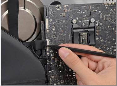
• Use the tip of a spudger to flip up the metal retaining bracket securing the camera cable connector to the logic board.
