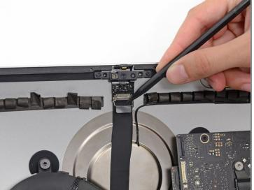
• Use the tip of a spudger to flip down the metal retaining bracket on the camera cable.
