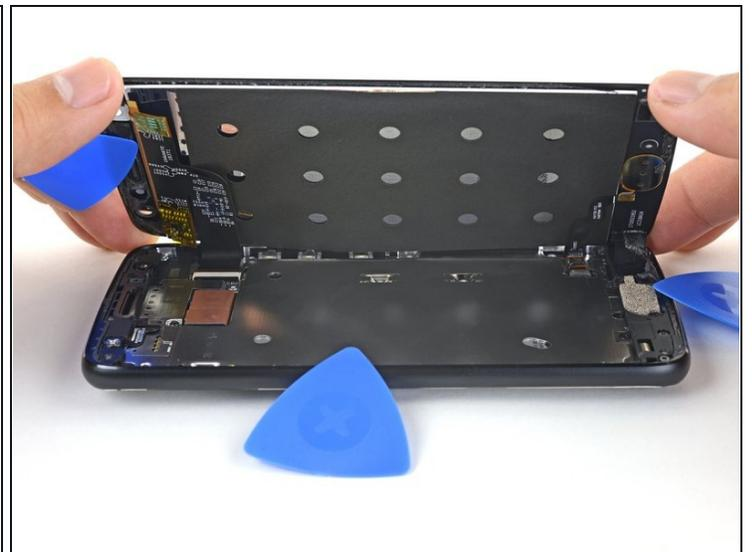
**⚠ Do not try to remove the screen yet—it is still attached to the phone by delicate flex cables.**
