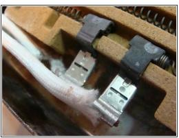
Install new cable ends and cable lugs.
