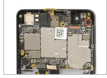
Take out the 4mm Phillips #00 screw, holding the mainboard to the frame.
