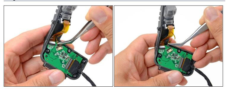
• Using your fingers or <u>tweezers</u>, gently pull out the backlight ribbon cable from its connector on the button board.
