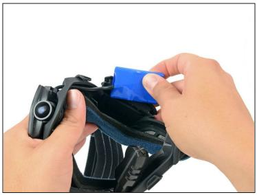
• Pull the battery out of its recess in the frame.
