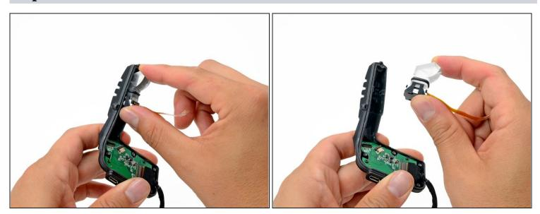
• Remove the viewfinder lens assembly from the viewfinder housing.
