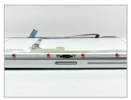
Remove the four small black Phillips screws along the top edge of the display.
