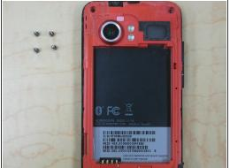
Remove 4 corner screws, you may have to remove a "VOID" sticker from one of the screw heads.
