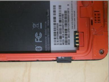
Depress MicroSD to eject it from the side of the case.
