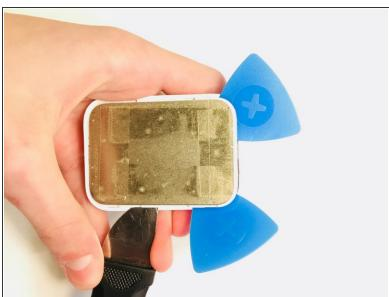
Carefully remove the clips on the side by pushing up with the Jimmy. If needed, use the plastic
