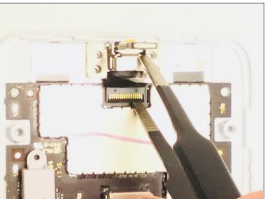
A similar adhesive can be found covering the plug for the lightning adaptor. Peel the adhesive back and gently lift the cable to disconnect the adaptor.
