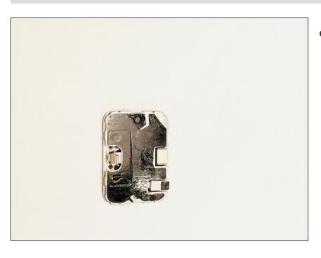
Remove the dock completely from the plastic frame.
