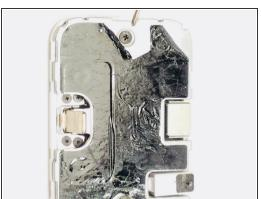
• The silver adhesive is covering two Phillips screws at opposite ends of the dock. Peel back the adhesive on these areas and remove both screws.
