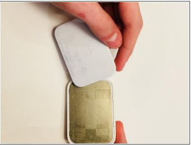
Take your <u>Jimmy</u> and push it in between the bottom cover and the body. Push down to lift the bottom cover.
