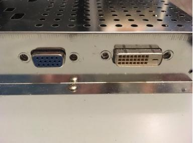
Remove the four 5mm nut screws.
