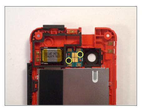
Remove two #000 Phillips screws attaching the Dual LED Flash board to the Rear Inner Frame.
