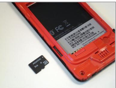
Pull the MicroSD card straight out of its slot.
