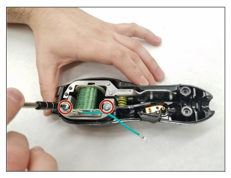
Remove two 23.0 mm JIS #1 screws attaching motor base to device body.
