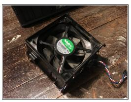
To take the fan out you have to pull the two tabs and pull the fan out.
