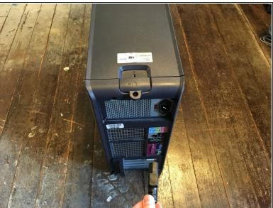
Power down your PC and remove the power cord from the back.
