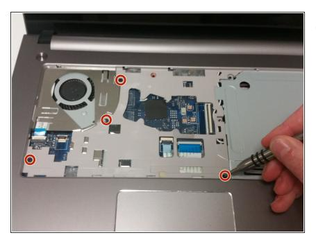
Remove four 7mm Phillips #1 interior screws.
